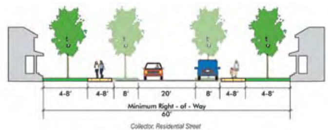
Figure 17: Sample Residential Collector Street Cross Section
