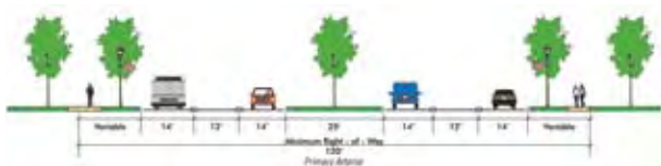
Figure 16: Sample Commuter Street Cross Section
