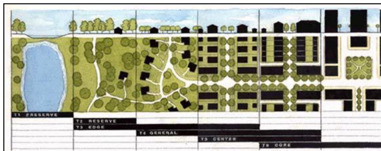
• Figure 7 - Urban Planners' Duany/Plater-Zybeck have written a model development code based on density rather than land use. From this they have developed a series of density zones, as opposed to land-use zones.
