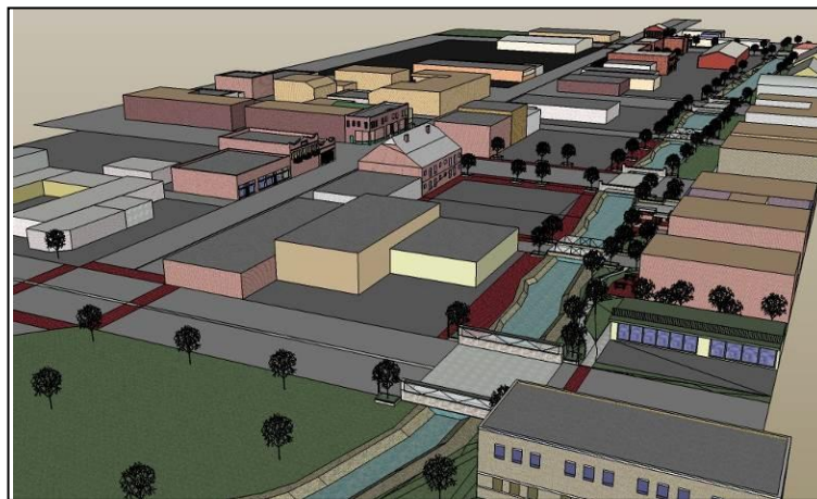
• Figure 15 - This concept drawing shows a functional drainage canal running down 7 th Street between Peoria and Rockford Avenues. The drawing illustrates how this drainage feature could serve as a catalyst for high-quality infill development
